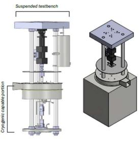
Testing materials at extremely low temperatures i.e arctic conditions, Liquefied: Natural Gas and Hydrogen)
