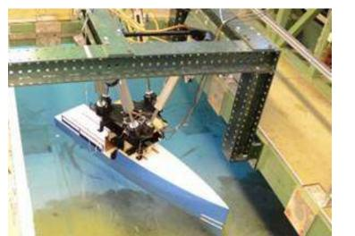
The Hexmove, or HexaPod is an electric operated model positioning device for model positioning and oscillation in six degrees of freedom. The Hexamove is used to position and oscillate models under the carriage in the towing tank while advancing with forward speed.
