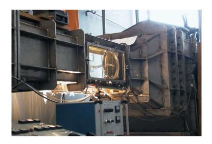
Test section dimensions: L x B x H =  $600 \times 300 \times 300 \text{ mm}$ 3;
